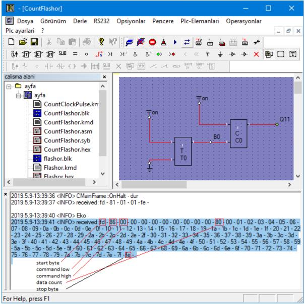
Fig.6: Verification of Echo Command in KUMANDA
