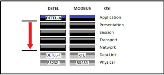
Fig.2: OSI Reference Model of the DETEL Serial Data Transmission Protocol
